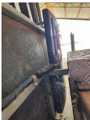
Example panel reader mounted on an auto-drafter
