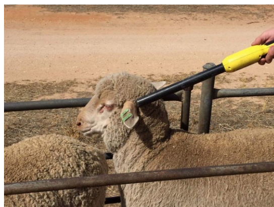
Example of stick reader scanning eID tag.
