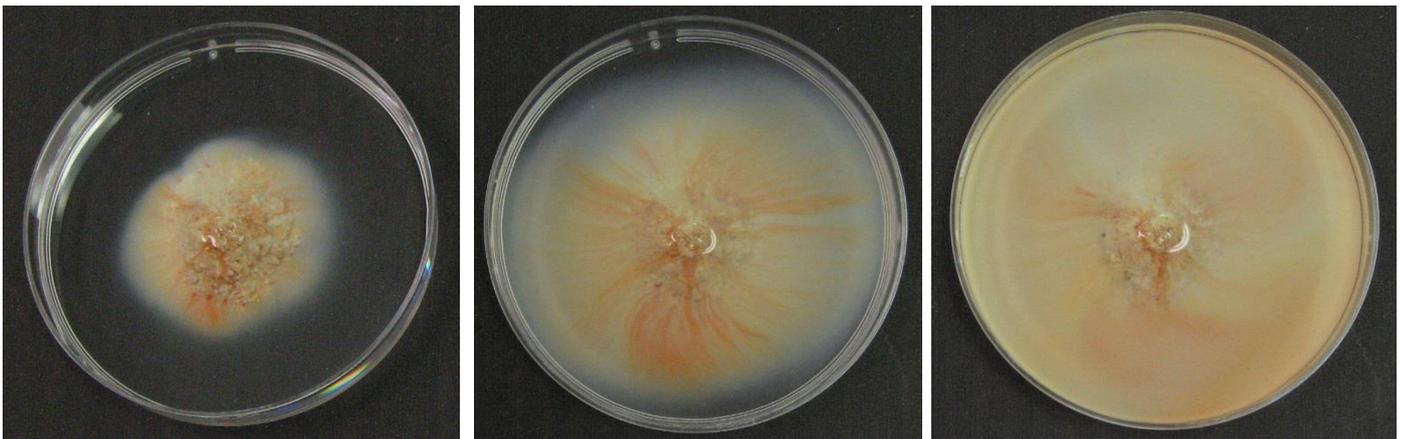
Figure 18. A slaking and highly dispersive clay sample from Cummins shown at 5, 30 and 120 minutes after placing in distilled water. Highly dispersive soils need to be treated with caution. Gain expert advice!
