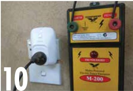
**10** We've covered the use of a similar device, the Belkin Wemo, back in *Farming Ahead* November 2014. It costs around \$60 and setup is very similar to the Arlec unit. It is controlled through the Wemo app (both Apple and Android platforms). Here we are using it to control an electric fence energiser.
