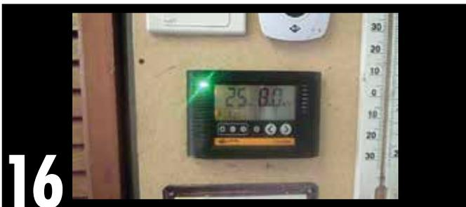
**16** Here we focused the Netcam on our electric fence control panel. The fence status can now be checked from anywhere with a smartphone or tablet. Gallagher does have a remote monitoring system for their i series energisers which will alert you to a low voltage situation, but it is a very expensive option. Note the Belkin Netcam cannot be used outdoors unless housed in a suitable weatherproof housing.
