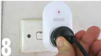
**8** Now you can plug your 240v equipment into the controller. It will handle a maximum current draw of 10 amps. Test the operation by switching it on and off through your device. The app will confirm whether the device has been successfully turned on or off. Several controllers can be added in a similar fashion and controlled through the app.
