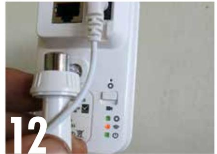
**12** To set up the camera, make sure you are in range of the wireless network the camera will be operated on. Plug the camera into a power outlet, and slide the rear switch up into the setup mode. If a wireless network is detected, the wireless LED should blink red.
