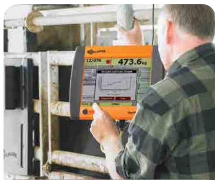
The TSi 2 weighs livestock and collects data for improved livestock management
